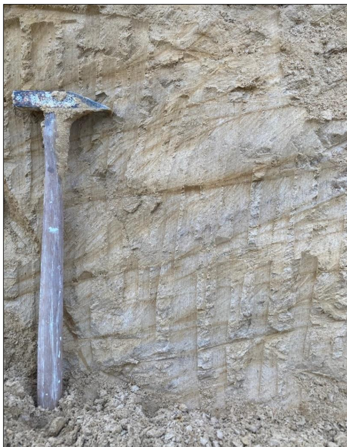
Figure 27. Cross-bedded silts and fine sands in a temporary exposure, Newport. Hammer is 0.3 m long.
