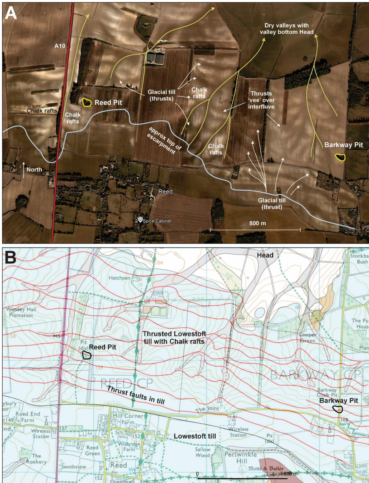
Figure 31. Glaciotectonics in the Reed-Barkway area. A. Aerial photograph showing paler chalk rafts interleaved with darker till sheets marking imbricate thrusts within the till. B. Interpreted geological map showing thrust faults within the Lowestoft Till Member.
