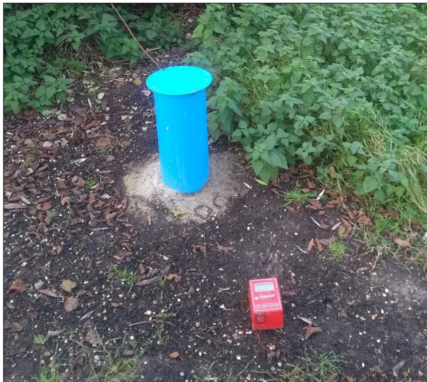
Figure 38: Tromino passive seismic instrument in operation next to an observation borehole.
