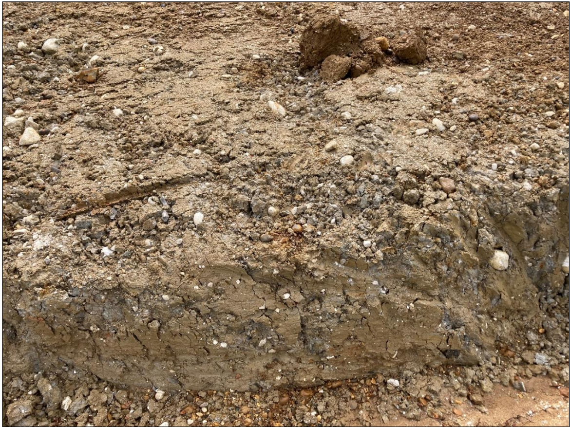
Figure 22. Typical Lowestoft Till Member, with many chalk fragments including well-rounded chalk pebbles in dark blue-grey clay. Plashes Farm section.
