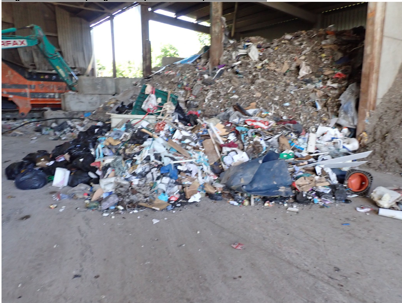
Image 3 shows waste spilling out of bay without 6m separation distance
